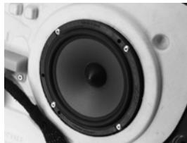
Focal speaker riveting (aluminum 4x16mm rivet).
