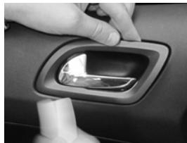
Use the supplied tool to remove the handle.
