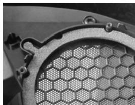
Remove the spikes that block the speaker positioning.
