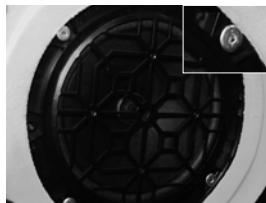
Cutting-out of rivets with a Ø 5,5/6mm metal drill.
